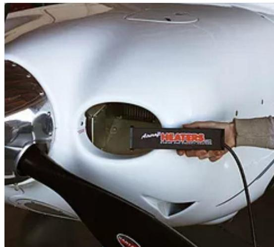
**Place two heavy moving blankets over the cowl or use an insulated cover and....**
